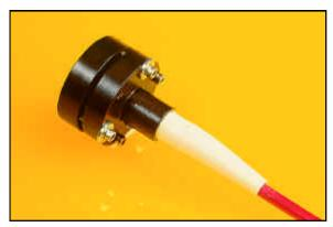
Fiber optic reflectors are used to reflect the light emerging from a fiber back in the reverse direction. They are used to build fiber interferometers, or with fiber fused splitters to measure backreflection within fiber optic components. They can also be used to measure the sensitivity of sources to backreflection from other devices, by providing reference reflection levels. This is very useful for deriving backreflection specifications for transmitters.
